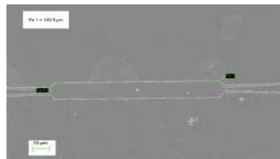
Figure 6. An image of fabricated SiOC based MMI with 100 μm of length
